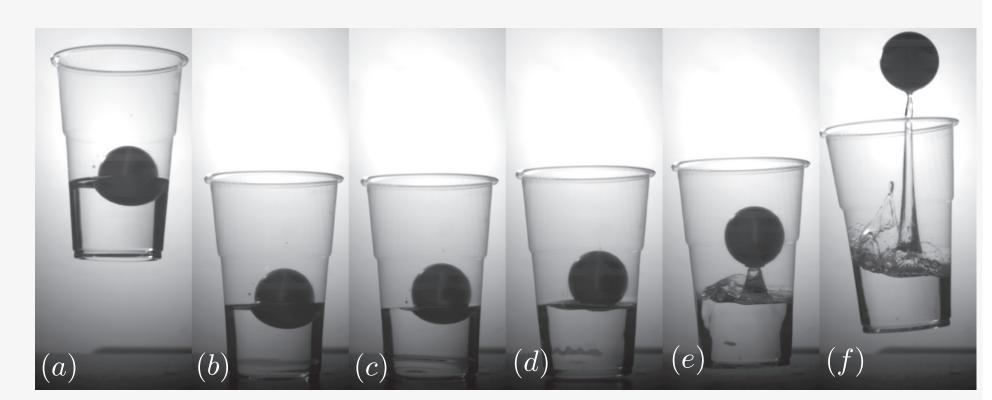
(Left, a–d) Experimental set-up. (Right, a–f) Series of pictures at t = 0 ms, 16 ms, 17 ms, 18 ms, 21 ms and 33 ms. Table tennis ball diameter is 40 mm.
