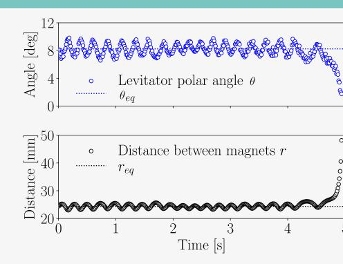
(Left) Snapshot of experiment. (Middle) Magnetic interactions (forces and torques) between the rotor magnet and the levitating magnet. (Right) Levitating magnet angle and distance, function of time (rotor freq.  $f = (216 \pm 2)$  Hz).
