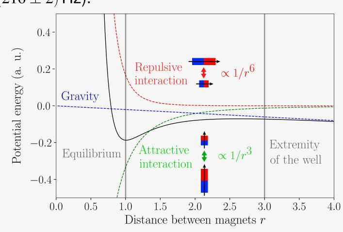
Potential energy (arbitrary units), function of the distance between magnets r, is sum of an attractive term  $\propto -1/r^3$  and a repulsive term  $\propto \theta/r^3$ . Since  $\theta \propto 1/r^3$ , the repulsive interaction potential energy is as  $1/r^6$ . The equilibrium position is at the minimum of the energy well, where small oscillations can take place. For a levitator below the rotating magnet, gravity leads to metastability
