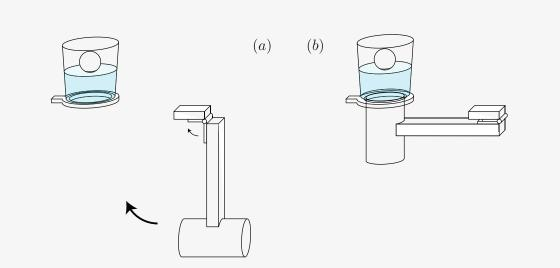
Control experiment using a pendulum as hammer > no ejection.
