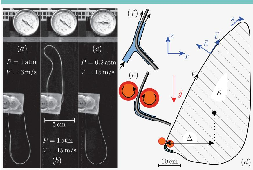
String loop entrained at speed *V* by two counter-rotating wheels (e) or air blown along a small segment (f) exhibits a transition from (a) a gravity dominated regime at low velocity towards (b) a self-supporting loop regime. (c) Reducing the pressure from atmospheric pressure to 20 kPa while keeping the high velocity reverts the string back to its lowered configuration.
