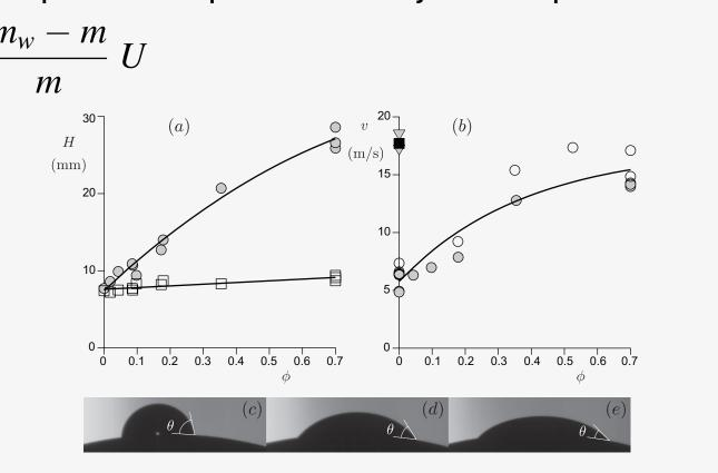
(a) Ball depth H function of ethanol fraction  $\phi$ . Circles: just before impact; squares: at rest. (b) Circles: Ejection velocity function of ethanol fraction  $\phi$ . (c) Drop spreading on ball,  $\phi = 0$ (water),  $\phi = 35 \%$ ,  $\phi = 70 \%$ .
