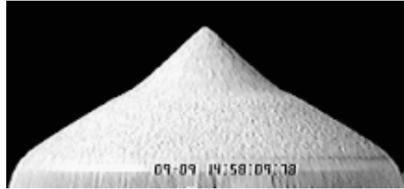
Fig. 2. – Snapshot of the flow for sand with coloured grains in the dense case. The exposure time of 1/50s allows to distinguish the grain velocities. The two regions, at a large angle with accelerating particles and at the small final angle with slow particles, are clearly visible.
