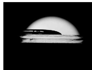
Fig. 9. Picture of a centimetric polymerized silicon drop taken from the side (about 0.5 mm thick).
