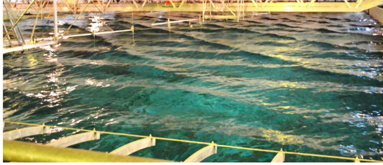
Fig. 2 View of the wave field in steady regime (after wave fronts) in resonant conditions with r = r_m and \varepsilon_1 = \varepsilon_3 = 0.14
