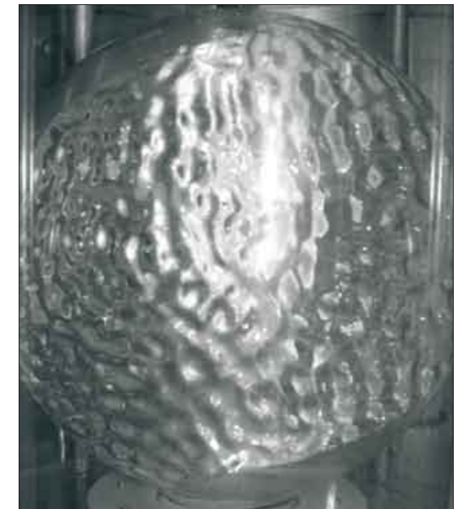
(Fig.1) Surface waves generated inside a spherical container made of glass during a parabolic flight. The fluid inside the sphere wets the surface and forms a layer along the inner boundary of the sphere. Waves are generated by vibrating the container.
