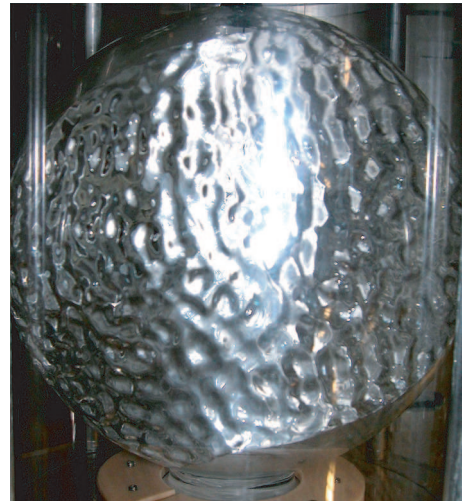
Fig. 3: (Colour on-line) Two-dimensional spherical subharmonic wave patterns under sinusoidal forcing at frequency f_0 = 30 Hz, and amplitude d_0 = 0.32 mm leading to a 1.16g acceleration. Spherical container filled with 20 cl of water.
