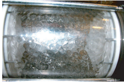
Fig. 2: (Colour on-line) Two-dimensional cylindrical subharmonic wave patterns (hexagons) under a sinusoidal forcing at frequency f_0 = 30 Hz, and amplitude d_0 = 0.29 mm leading to a 1.06g acceleration. Cylindrical container filled with 30 cl of ethanol.
